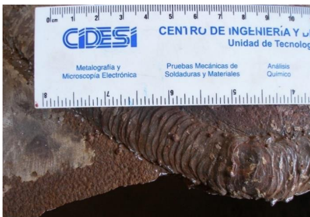
Figure 3 The image shows the right area of the crack. There is seen the change in crack growth from the weld toe to the body of the pipe
