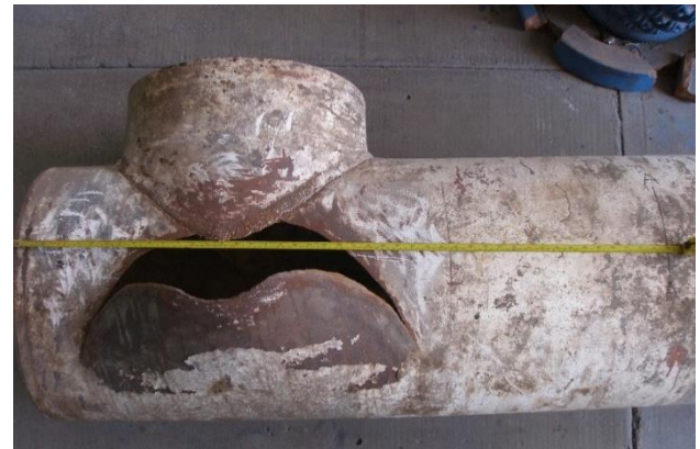
Figure 1 The image the connection type "T" in the condition of delivery to the laboratory. Note the fracture and coating on the external surface
