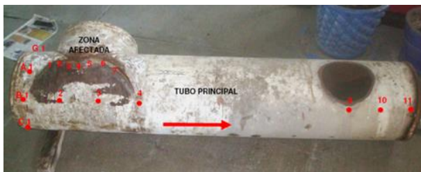
Figure 6 The image shows the regions where the thicknesses measurements were carried out Source: Own work
