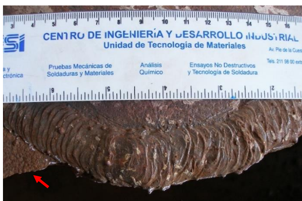
Figure 2 The image shows the fracture zone in the region of the weld
