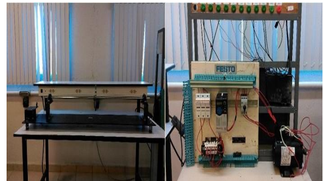
Figure 1 Rotodynamic system and PowerFlex 525 driver Source: UNACAR mechatronics laboratory facilities
