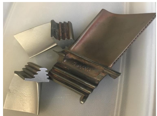
Figure 2 Two rotor blades of an axial compressor and a power turbine blade
