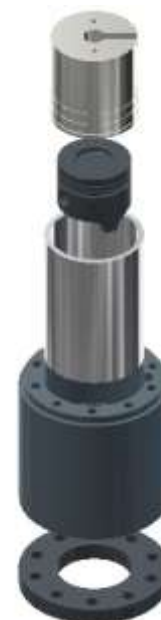
Figure 6 Exploded view of the virtual assembly of the device for fatigue and compression tests for gasoline engine pistons Source: Self Made
