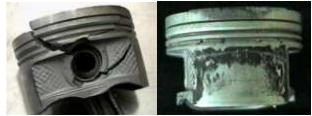
Figure 2 Piston damage due to fatigue and wear Source: Self Made
