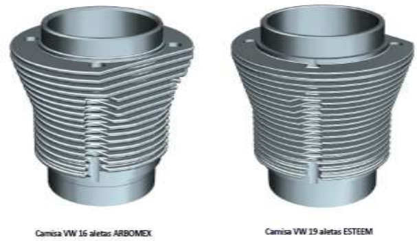
Figure 1 16 and 19 fin shirts, respectively Source: Own Elaboration [CAD Software]
