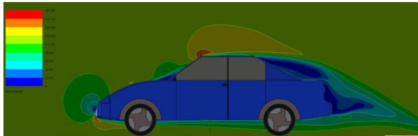
Figure 15 Results of the velocity contours of Model B with 5744807 cells in the mesh
