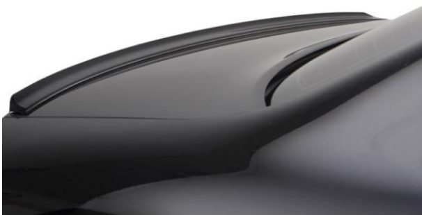
Figure 3 Design of a lip type spoiler Source: Own elaboration in Solidworks
