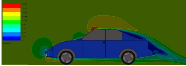
Figure 14 Results of the velocity contours of Model A with 5744807 cells in the mesh
