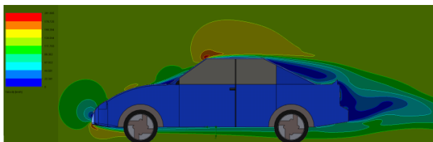
Figure 19 Results of the velocity contours of Model F with 5744807 cells in the mesh
