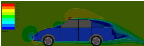
Figure 15 Results of the velocity contours of Model B with 5744807 cells in the mesh
