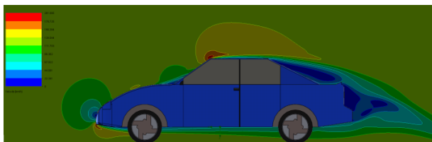
Figure 17 Results of the velocity contours of Model D with 5744807 cells in the mesh
