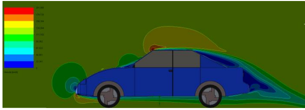
Figure 14 Results of the velocity contours of Model A with 5744807 cells in the mesh
