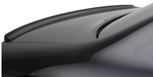
Figure 3 Design of a lip type spoiler Source: Own elaboration in Solidworks
