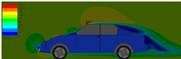
Figure 16 Results of the velocity contours of Model C with 5744807 cells in the mesh
