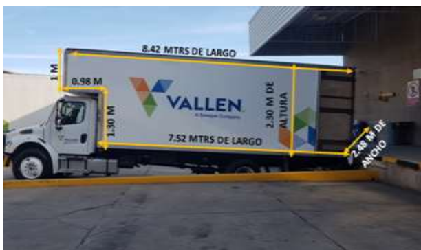
Figura 2 Image of the external dimensions of the Load Unit Source: Self Made
