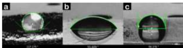
Figure 6 Contact angle of zinc oxide nanostructures. a) powders, b) thin film and c) nanowires
