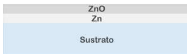
Figure 3 Architecture of the PVD-synthesised thin film
