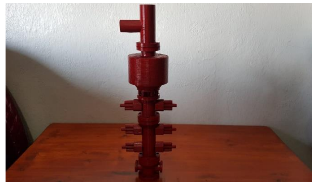
Graphic 17 Double and single ram socket with spool and waterline. Source: Author's contribution (October 2021)
