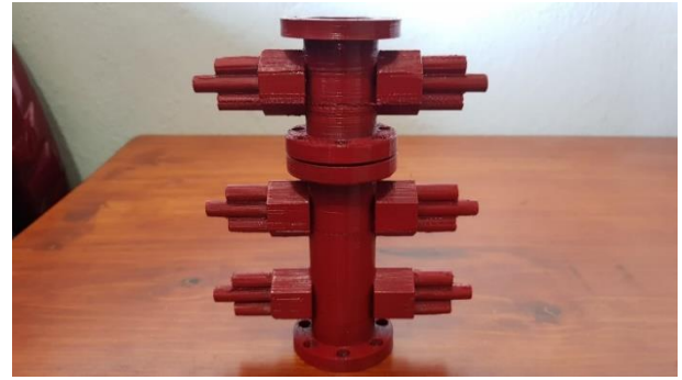
Graphic 14 Double and single ram socket Source: Author's contribution (October 2021)
