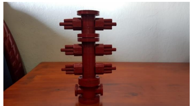
Graphic 15 Double and single ram socket with spool Source: Author's contribution (October 2021)
