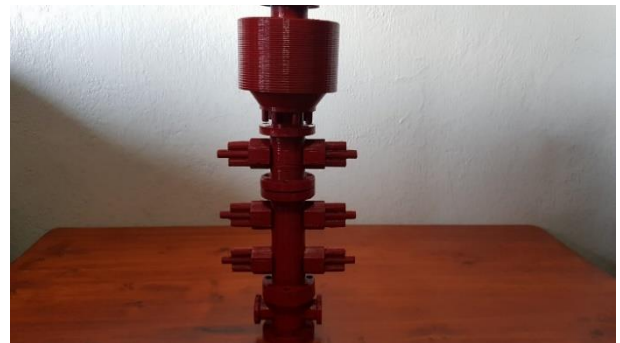
Graphic 16 Double and single ram socket with annular preventer spool Source: Author's contribution (October 2021)
