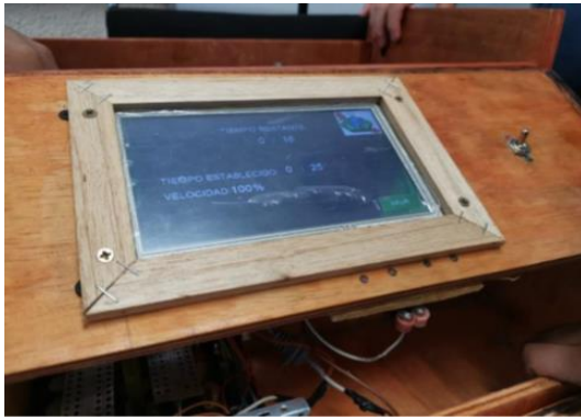
Figure 6 In-dash touch screen installation Source: (own elaboration,2020)
