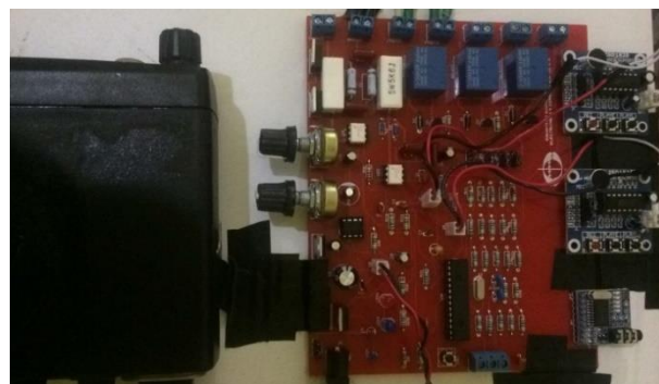
Figure 5 Modules incorporated into the electronic card connected to the radio station for transmission with Motorola EP450 equipment
