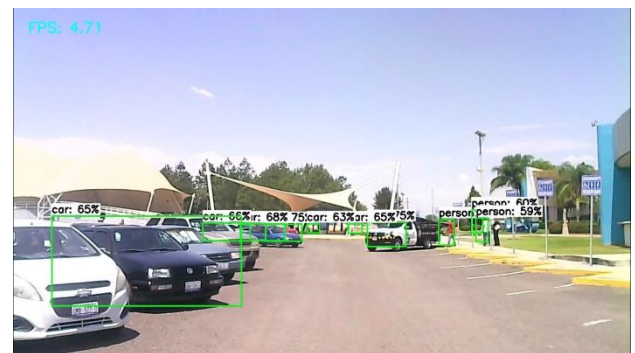
Figure 4 Field test of the basic car-mounted detection system, showing the detection of people and cars
