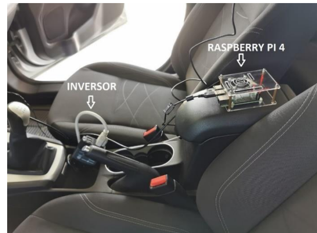
Figure 2 Raspberry Pi 4 board mounted inside the cabin of the car and powered by an inverter connected to the battery
