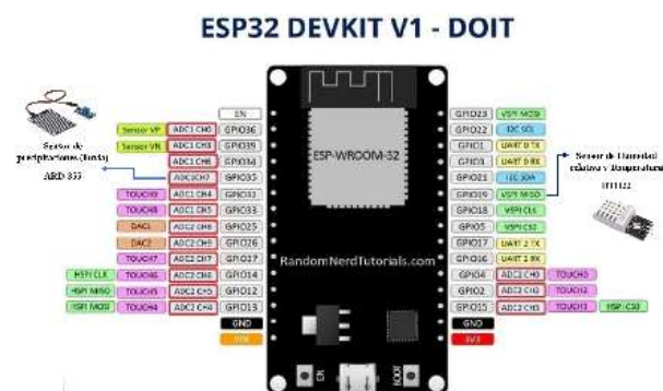
Figure 5 Schematic diagram of sensors with connection to the ESP32 microcontroller
