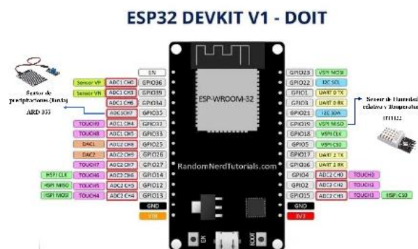
Figure 5 Schematic diagram of sensors with connection to the ESP32 microcontroller
