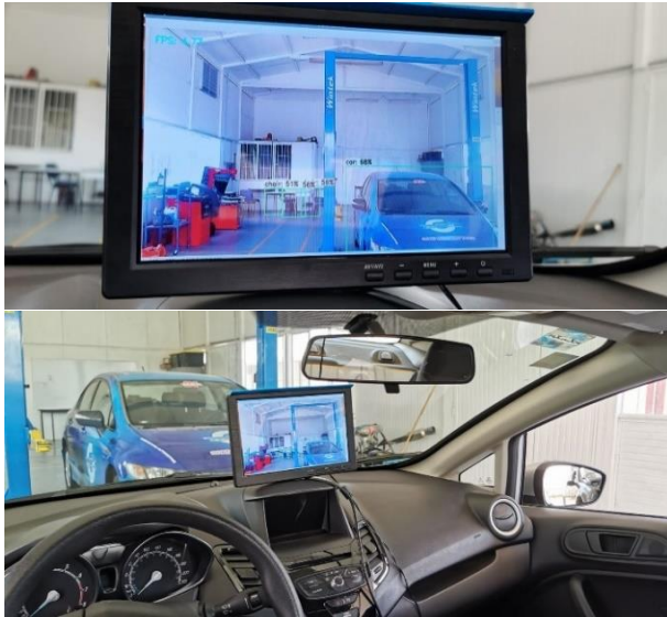
Figure 3 In-dash colour LCD screen, which displays real-time pedestrian detection on the road and corresponding alerts
