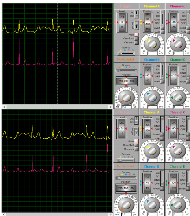
Figure 24 ECG lead I signal displayed on oscilloscope (yellow) and ECG signal after filtering squared (magenta) Source: Own elaboration
