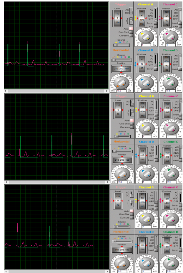
Figure 25 ECG signal after filtering squared (magenta) and comparator output (green). Oscilloscope at 0.2 seconds per division. Source: Own elaboration
