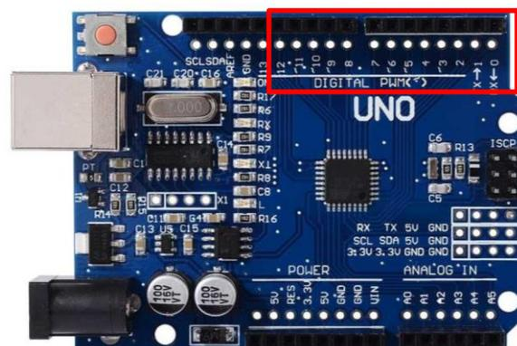
**Figura 2** Tarjeta Arduino Uno Inputs/Outputs
