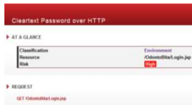
Figura 4 Vulnerabilidad (VI 1 ) “Cleartext Password over HTTP”
