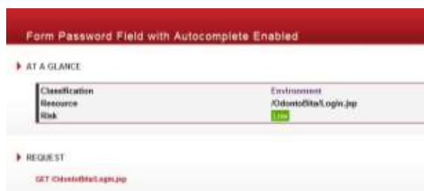
Figura 5 Vulnerabilidad (VI 3 ) “Form Password Field with Autocomplete Enabled”
