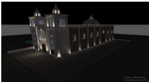
Figure 11 Rendering of the lateral façade of the proposed luminaire of the Basílica Menor de Nuestra Señora de Guadalupe, "La Villita", elaborated with the DIALux program
