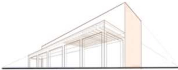
Figure 7 Composition of wooden beams in the archetypal colonnade. Two-point perspective representation on the section of wooden beams in colonnade porches, where the structure is marked up to the midpoint of the entire porch section, highlighting the critical point
