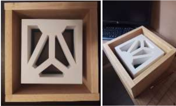
Figure 6. Negative mould made Source: Own elaboration, Dalia Cruz Martínez 2022
