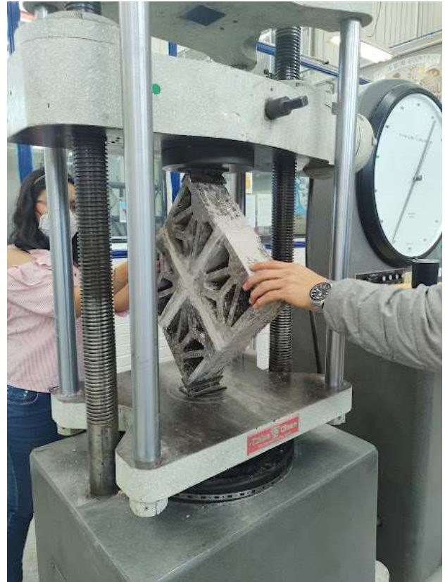
Figure 11 Laying of the wall in a universal machine. Source. Own elaboration, Dalia Cruz Martínez 2022
