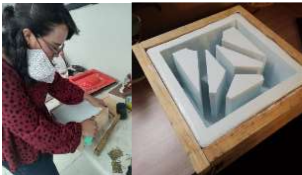
Figure 7 Final positive mould Source: Own elaboration, Dalia Cruz Martínez 2022.
