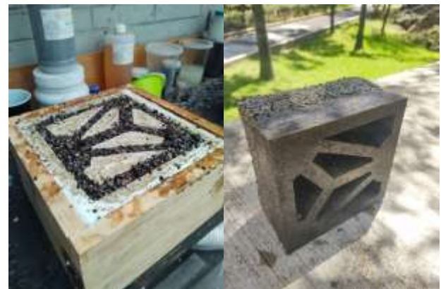
Figure 8 Pouring of aggregates and final result Source: Own elaboration, Dalia Cruz Martínez 2022
