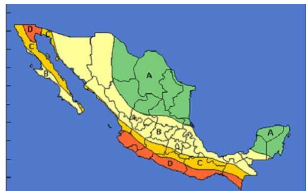
Figure 9 Seismic regionalization in Mexico Source: Manual for the design of civil works, earthquake design, Federal Electricity Commission (C.F.E.), 1993
