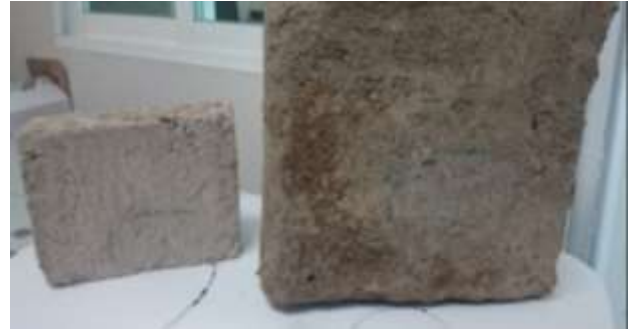
Figure 10 Adobe bricks from the southeastern of Mexico (half scale) and from central part of the country (full scale)
