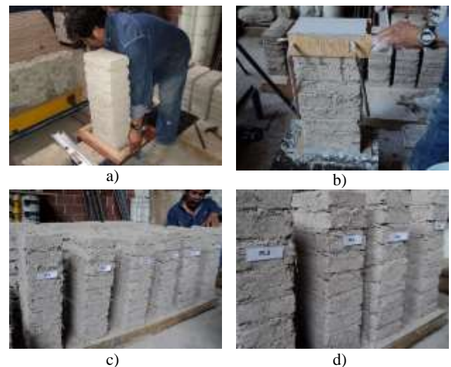
Figure 7 Specimens built for compressive tests: a) construction of pillars; b) planar surface for performing a uniform stress distribution; c) storage of pillars; d) numbering of pillars Self-authorship
