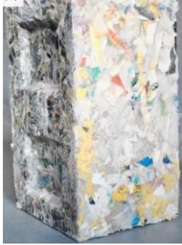
Figure 7 PET bricks Source: Ecologiaverde , November 22nd, 2017
