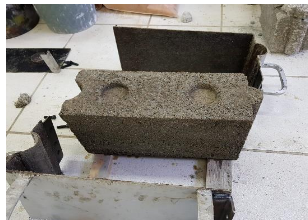
Figure 15 Eco-friendly masonry piece for non-structural walls
