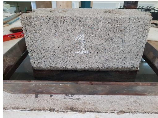
Figure 18 Maximum initial absorption test of the ecological part
