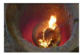
Figure 3 Cast aluminum cans to a Temperature of 700  $^\circ C$
