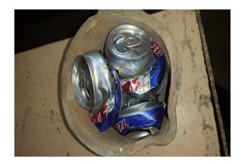
Figure 2 Clay pot for casting
