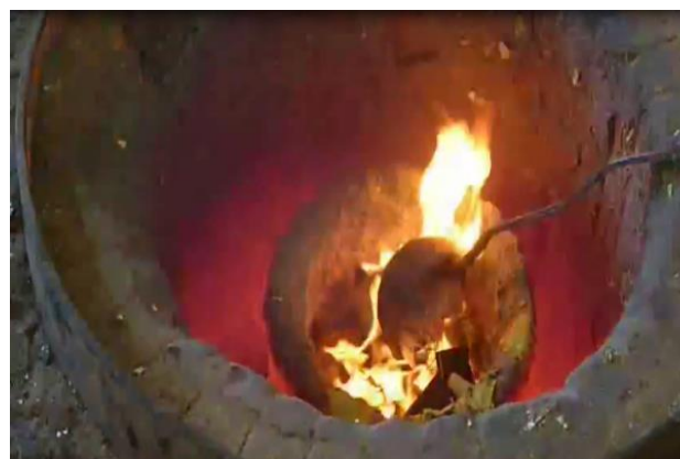
Figure 3 Cast aluminum cans to a Temperature of 700 °C
