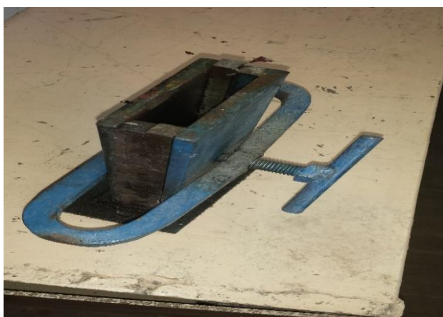
Figure 1 This is the permanent mold or chaponera for the emptying
