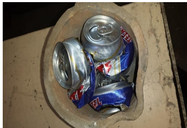
Figure 2 Clay pot for casting
