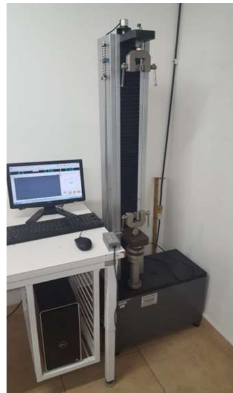
Figure 4 Tension, bending and compression machine model: WDW-S5
