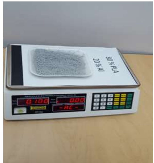
Figure 1 Mixture of PLA with metallic aluminum powder (80% PLA and 20% Al). Source: TecNM / ITN
