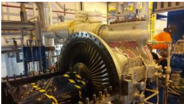
Figure 1 Blade rotor of compressor gas turbine Note. Adapted of Compressor turbine disk, Villagrán-Villegas Luz Yazmin, 2017
