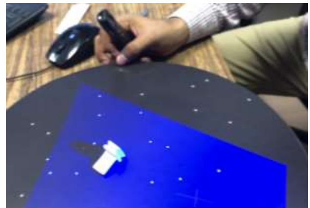
Figure 5 3D digitization process of blade. Note: Adapted "Study of wear damage in compressor turbine blades"(p. 76), Villagrán-Villegas L. , 2017
