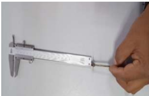
Figure 22 Nozzle height determination Own authorship
