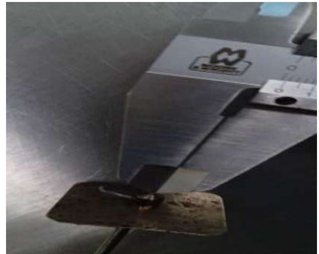
Figure 20 Determination of the outer diameter of the nozzle
