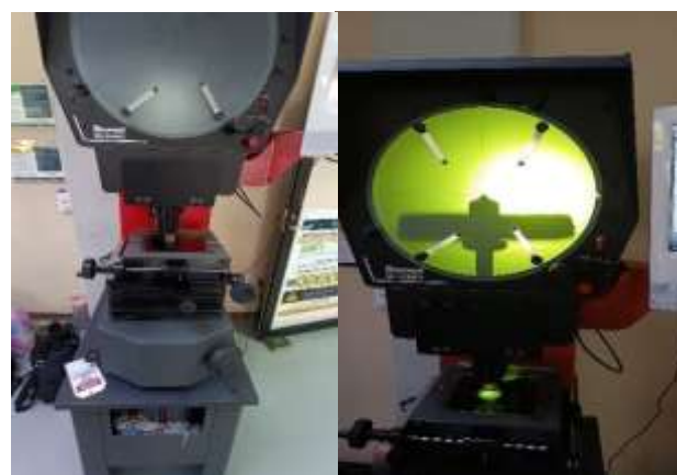
Figure 33 Obtaining geometries with optical comparator Own Authorship
