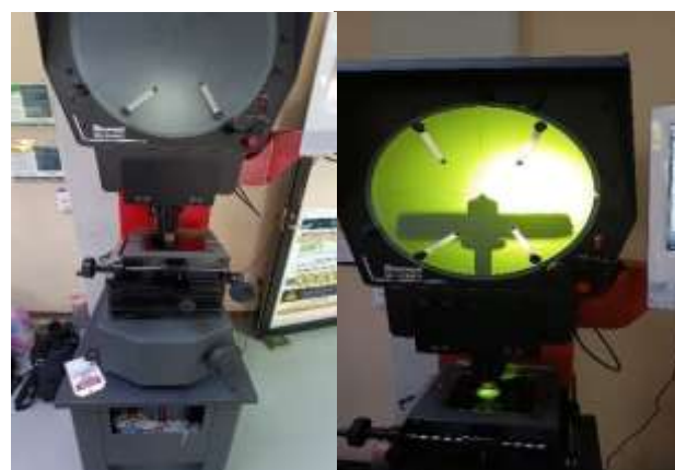
Figure 33 Obtaining geometries with optical comparator Own Authorship
