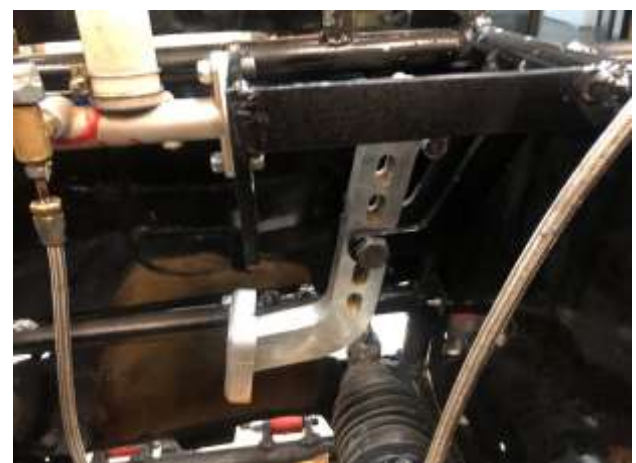
Figure 23 Baja SAE 2023 Vehicle Mounted Pedal
