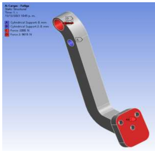
Figure 11 Global view of the pedal representing loads and supports exerted on the model for study
