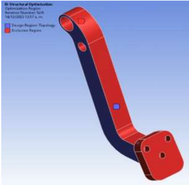
Figure 16 Global view of the pedal representing topological region (blue A) and exclusion region (red A)
