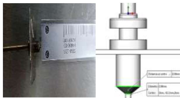
Figure 27 Obtaining the conical part of the nozzle Own Authorship
