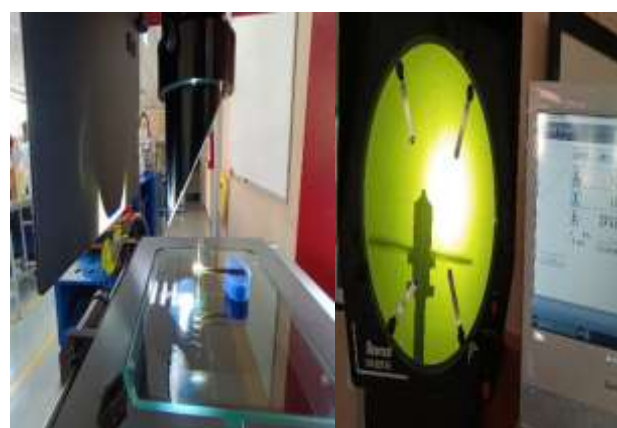
Figure 34 Obtaining nozzle geometries Own Authorship
