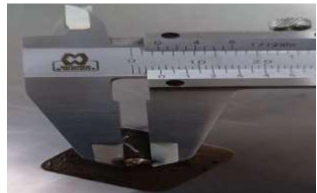
Figure 21 Obtaining the general diameter of the nozzle
