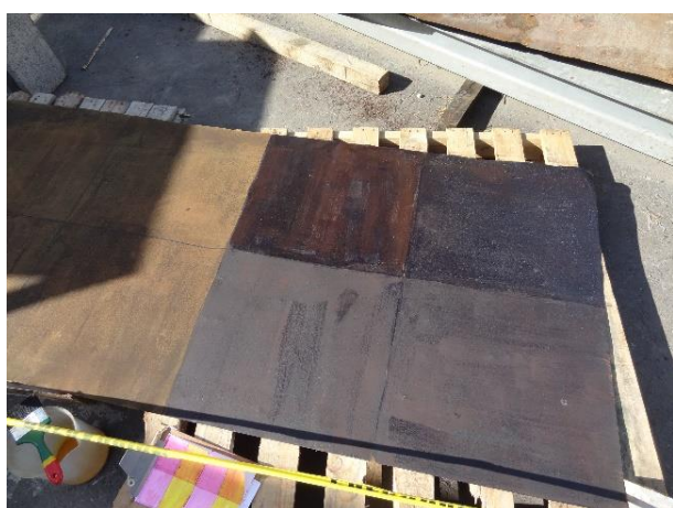
Figure 8 Beginning of converter application by sections on sample sheet with oxide present (15:07 PM)
