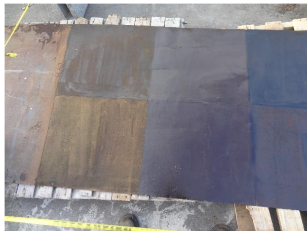
Figure 9 With sections of converter application on sample sheet with presence of oxide (16:49 PM)
