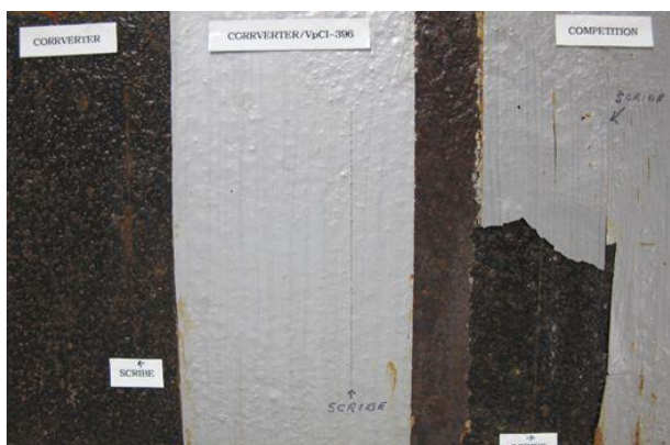
Figure 1 Salt fog test Source: CORTEC Corporate
