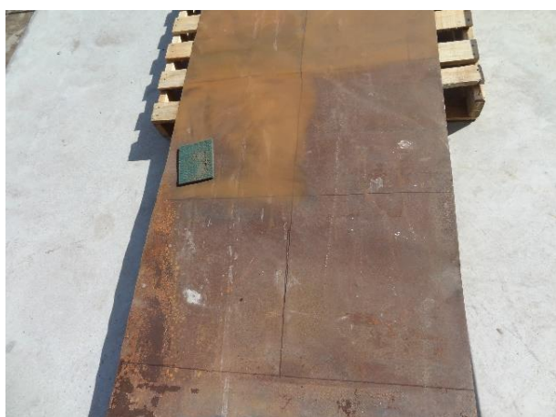
Figure 7 Cleaning of sample sheet with presence of rust (10:00 AM)
