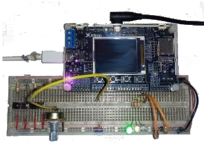
Figure 15 The green led turns on when the potentiometer exceeds the programmed level
