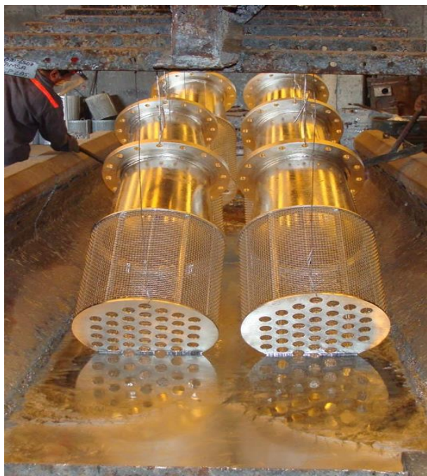
Figure 4 Galvanized parts over molten zinc Source: Metalyzinc Quality
