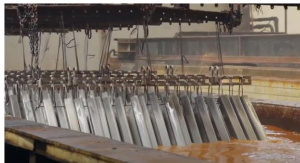
Figure 3 Steel in salt bath Source: Ruiz, E. (2016) Practical guide for hot dip galvanizing. Retrieved from https://www.idu.gov.co/web/content/7423/guia_galvanizado_24nov14+(1).pdf
