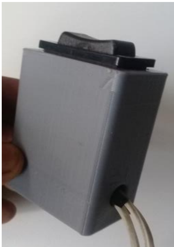
Figure 17 3D Printing in PLA. Switch housing Source: own
