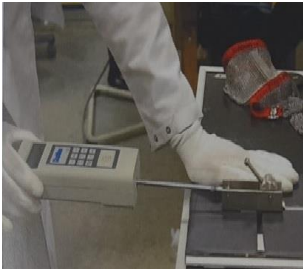
Figure 2 Adhesion test Dynamometer Source: Own elaboration
