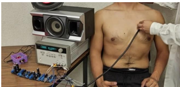
Figure 15 Test carried out on a subject, after physical activity, using a Sallen-Key fourth-order active low-pass filter
