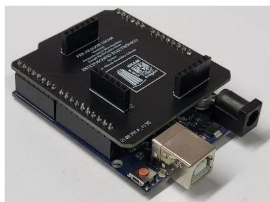
Figure 12 Printed circuit board for the connection between the Arduino uno and the modules AD8232, RTC-DS3132, microSD card reader
