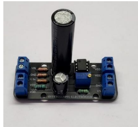
Figure 8 Electronic circuit board with the passive elements of the second order active low-pass filter to be assembled to the preamplifier and the speaker
