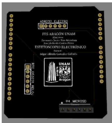
Figure 10 3D printed circuit board for connection between Arduino uno and AD8232 modules, RTC-DS3132, microSD card reader
