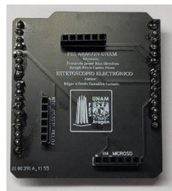
Figure 11 Printed circuit board for connection of AD8232, RTC-DS3132, microSD card reader modules
