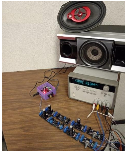
Figure 15 Experimental arrangement integrated by modules of the filters using and of the audio amplifier
