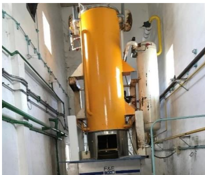
Figure 4 Ice tube machine in the Hielo factory
