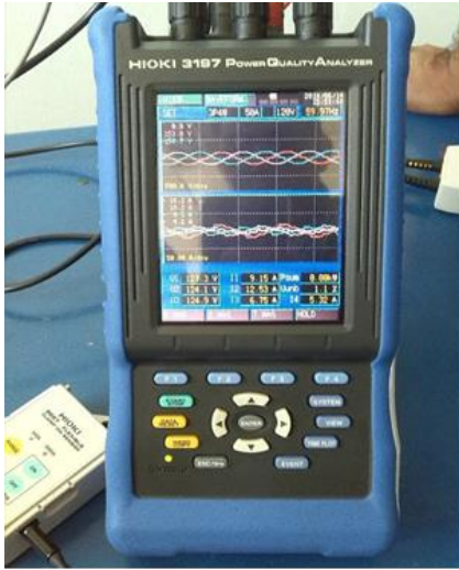
Figure 8 Appreciable current unbalance in phase 2 (V2)
