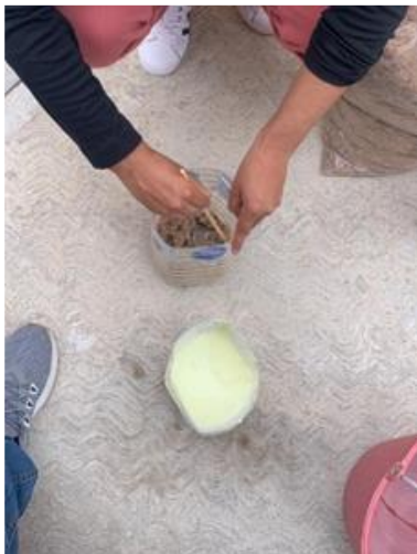
Figure 15 Mixing of cardboard with Resistol 950. The mixture is mixed little by little to make it more homogeneous Source: author's own work, 2022
