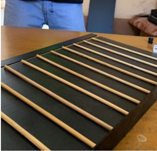
Figure 14 Construction of the mould, the texture seeks a good performance in the face of the plaster Source: own authorship, 2022
