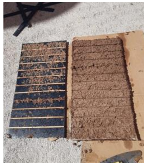
Figure 17 With the help of a spoon, the mould can be removed from the cardboard plate Source: own authorship, 2022
