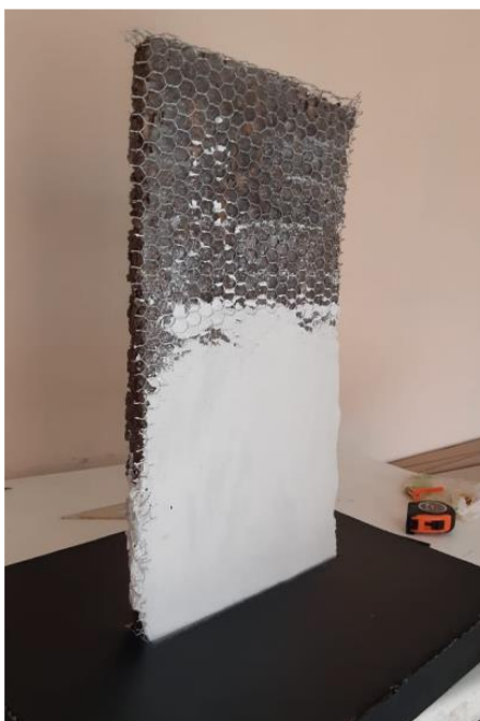
Figure 19 The different layers of the panel can be seen. The first layer or core is compressed cardboard, the second layer is mesh and finally there is the gypsum sheathing
