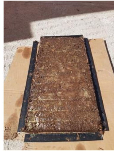
Figure 16 Placing the mixture inside the mould Source: own authorship, 2022
