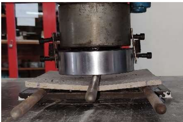
Figure 7 Attachment and arrangement for bending test (NMX-C-234-ONNCCE-2015)
