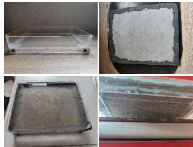
Figure 9 Performance of permeability test on control specimen (control)
