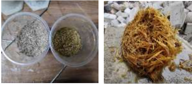
Figure 2 BC saturated in water and subsequently impregnated with sodium silicate
