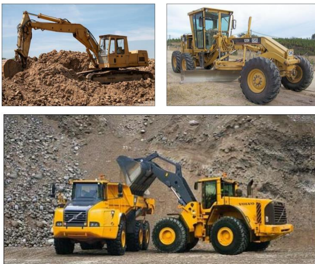
Figure 2 Excavator, Motor Grader, Loader and Dump Truck
