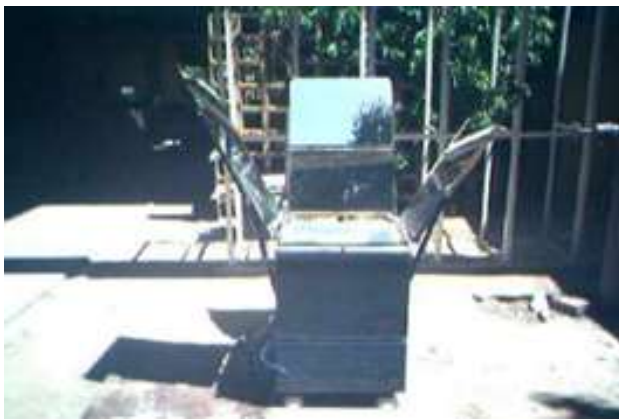
Figure 1 Box-type solar stove
