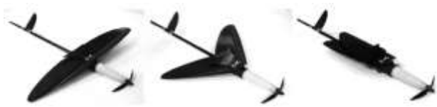
Figure 4 AquaMAV fuselage inspired by sulidae birds Siddall, R. et. al. (2017)
