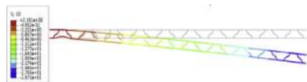
Figure 7 Bending of the clad corrugated surface based on the thin elements of the beam Ermakova, A. et. al. (2017)
