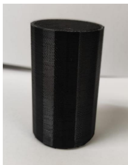
Figure 7. Straight circular cylinder printed on Ender 3 Pro 3D printer Source: Own elaboration
