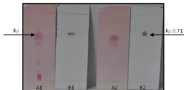
Figure 2. Thin layer chromatography of the semi-purified (A1 and B1) and purified (A2 and B2) extract developed with ninhydrin (A1 and A2) and with 10% cupric sulphate in 8% phosphoric acid (B1 and B2)
