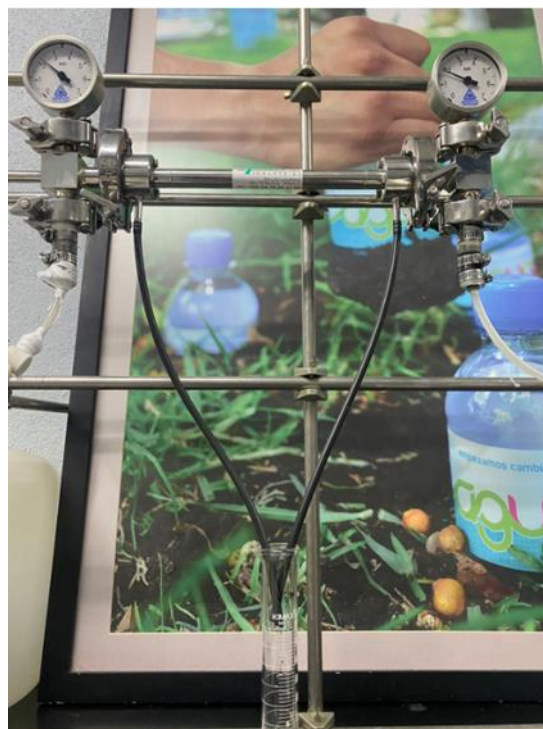
Figure 5 Membrane permeates for sampling
